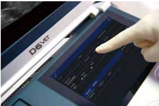
8-inch high-sensitivity touch screen that can be operated while wearing sterile gloves
