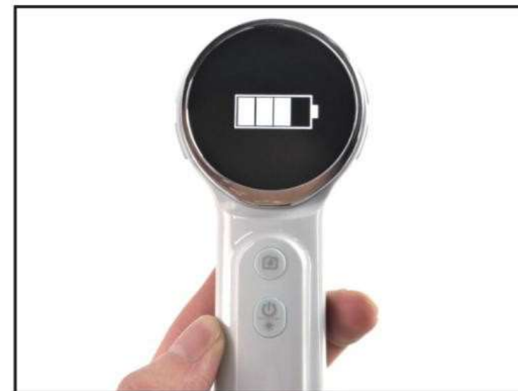
Shutdown charging status
