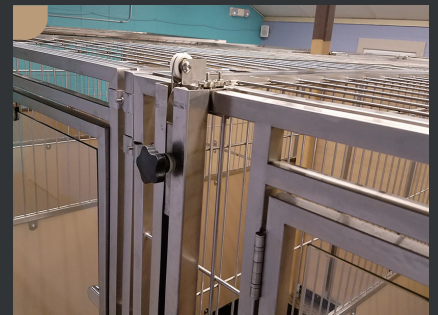
Control knob of the double control pulley system with weight balancer
